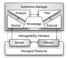
Figure 1: Autonomic computing control loop
