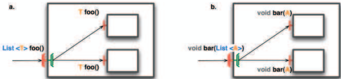
Figure 3.3. Comparison of signatures of methods between client multicast interfaces and server interfaces.
